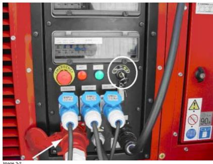
Image 3-2 Contact key and power cable of pump
